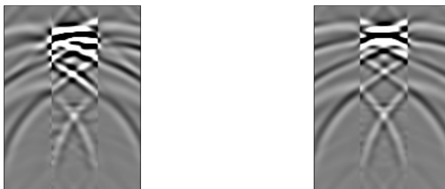
Figure 3: left) Fluid layer embedded in the solid; left and right interface conditions differ (right one is correct). right) Modified interface condition (as sketched in Figure 2) leads to accurate results
